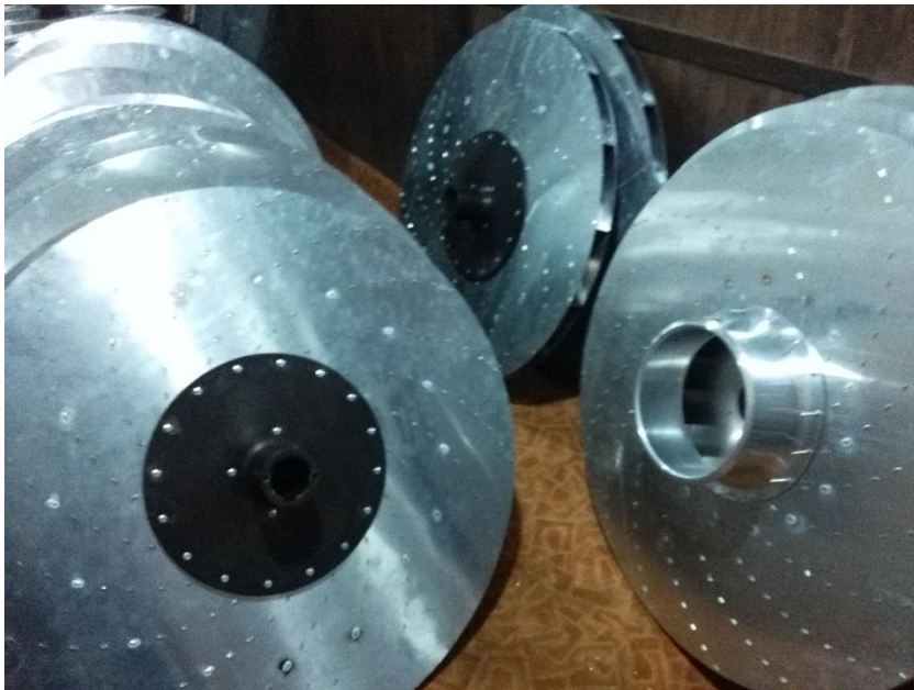
FINAL ASSEMBLY FAN maximum diameter 994mm
