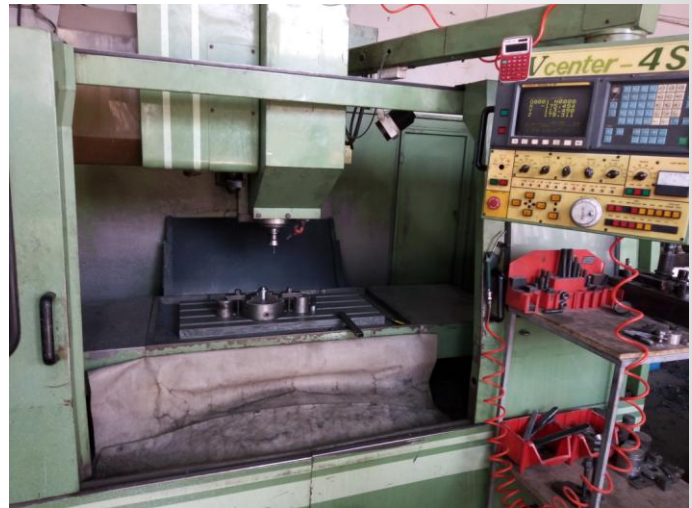
CNC MILL TYPES BEMATO CONTROL FANUC O-MD & V CENTER-4S (X=650mm,Y=380mm,Z=460mm)
