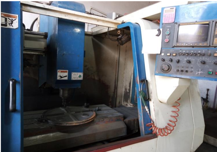
CNC MILL TYPES BEMATO CONTROL FANUC O-MD & V CENTER-4S (X=650mm,Y=380mm,Z=460mm)
